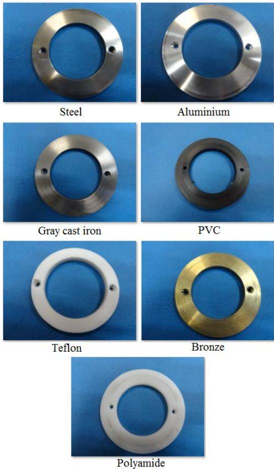
**Figure 4.** The disc pads of the friction couple
