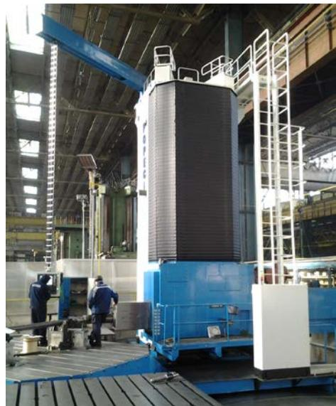
**Figure 15:** Textile guards used for the protection of Y axis guideways on an AFP type machine
