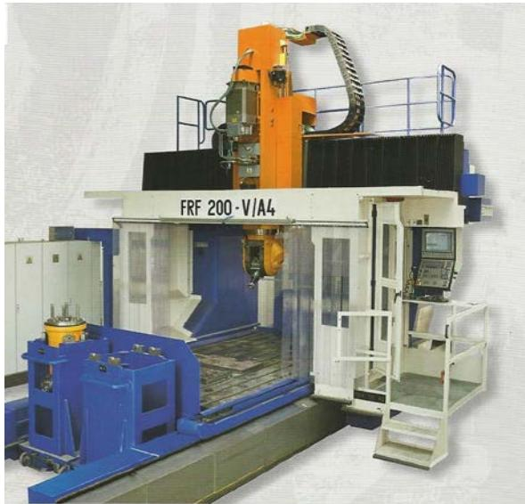
**Figure 14:** TOS KURIM milling machine with traverse guideways protected by textile guards
