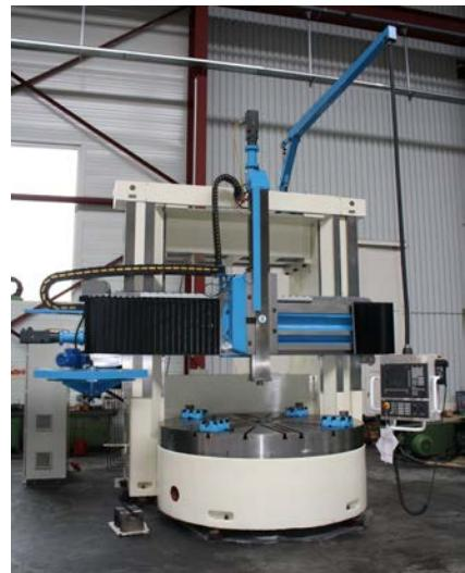
*Figure 10: Textile guards used for cross rail of a vertical lathe GPM make*
