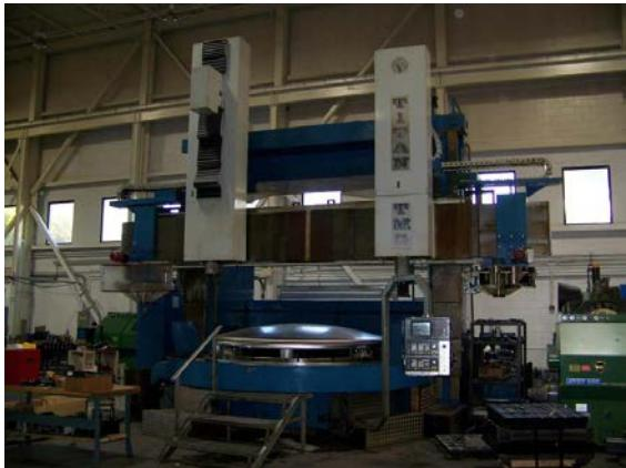
**Figure 12:** Vertical lathe TITAN make; left side has the guideways protected with guards on textile support
